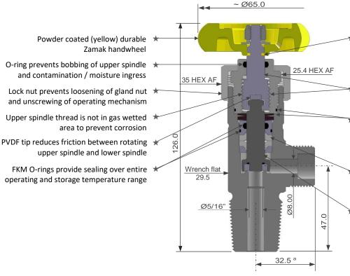
Upper spindle designed to shear from failure groove to prevent damage to the operating mechanism in case excessive torque is applied
